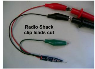
At QRP power levels, shielding is not a requirement. If holding the probe by the leads is not acceptable, a plastic tubing enclosure or clear shrink sleeving will do the job quite nicely.
